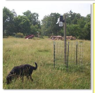
**LEFT:** The temp/humidity sensor is at an ideal height over representative ground cover. The rain gauge is at a good height to avoid dog-watering by the "Weather Lab."
